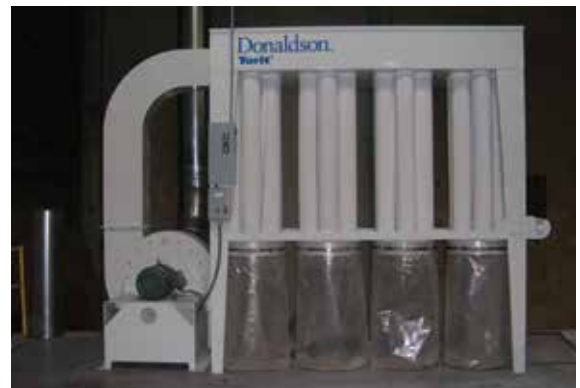
IRD - Wood Shop 5,000 cfm (8,493 m 3 /h)
