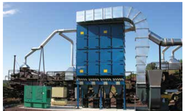
DLMC on Rock Crushing 41,000 cfm (69,645 m 3 /h)
