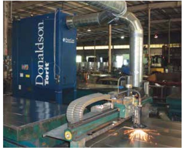
TG on Plasma Cutting 3,400 cfm (5,775 m 3 /h)
