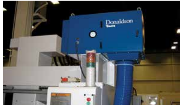
DMC on Wet Machining 390 cfm (662 m 3 /h)
