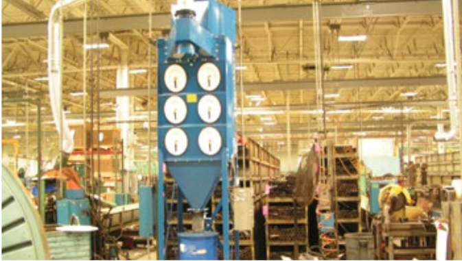
DFO 3-6 on Sawing of High Pressure Hydraulic Hose
