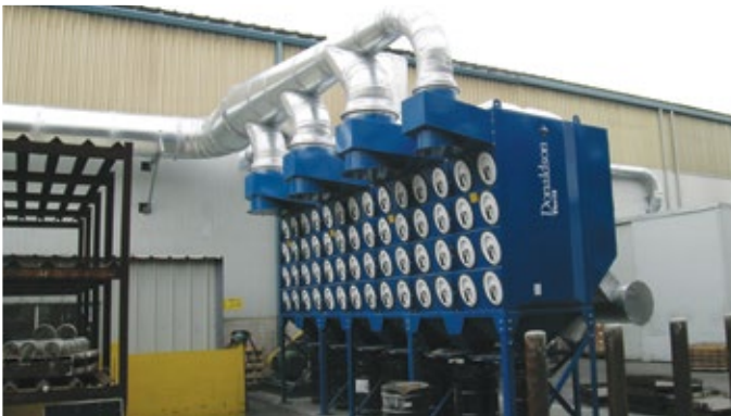
DFO 4-112 on Titanium Grinding
