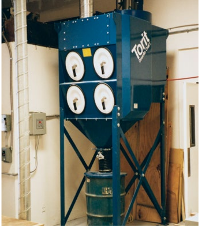
DFO 2-4 on Fiberglass Routing & Cutting
