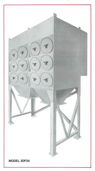
**Directional downflow** of contaminated air, assisted by gravity, minimizes re-entrainment of dust dislodged by cleaning pulse of 90 psig compressed air.
